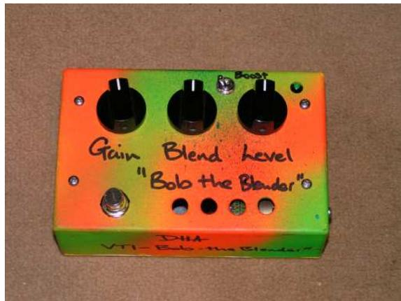
The VT1 "BtB" has a built-in voltage doubler circuit; this generates 24V from the existing 12V power supply. The 24V is used to supply the anodes or plates of the valve.
