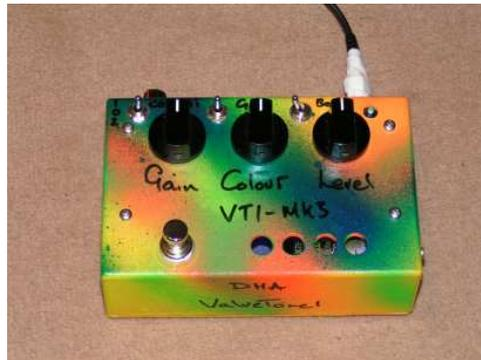
The ValveTone 1 MK3 is fitted with 2.1mm external PSU adaptor for use with a 12v @ 1200mA external supply. The user should use a well regulated external supply as the better the regulation then the less the hum when at higher gain levels. The inner of the connector is the positive, there is reverse polarity protection so no harm will be done if you get it wrong. There is an internal switch mode power supply which doubles the 12V to 24V for the valve anodes or 'plates'.
