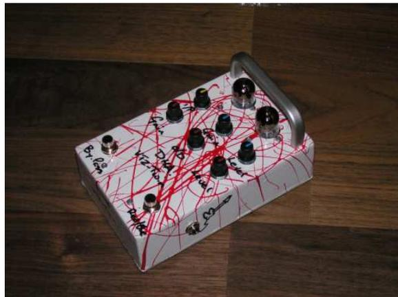
The VT2-Twin-Bass has two built-in voltage doubler circuits; this generates 24V from the existing 12V power supply. The 24V is used to supply the anodes or plates of the valves, two are used to ensure good power supply decoupling between channels.
