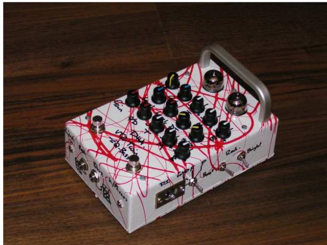
The VT2-Twin-EQ-Bass has a two built-in voltage doubler circuits; this generates 24V from the existing 12V power supply. The 24V is used to supply the anodes or plates of the valves, two are used to ensure good power supply decoupling between channels.
