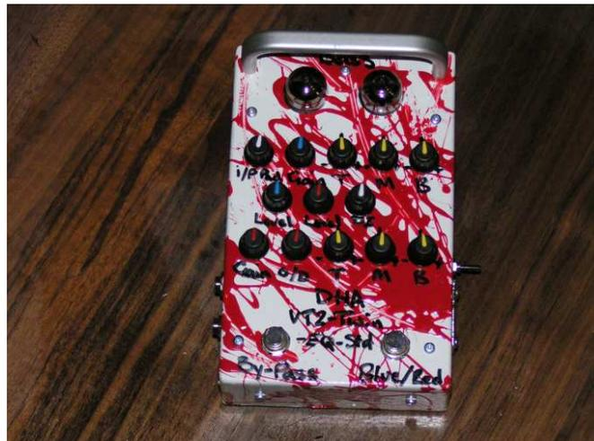
The VT2-Twin-EQ-Std-Bass has a two built-in voltage doubler circuits; this generates 24V from the existing 12V power supply. The 24V is used to supply the anodes or plates of the valves, two are used to ensure good power supply decoupling between channels.
